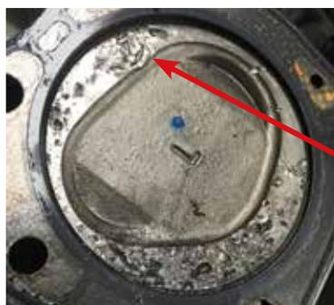
*A piece of old piston ring between the piston and head can destroy both!*
