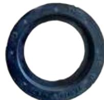
*Injector Seals must be fitted with this side up, to a depth between 0 - 0.4mm from the top face.*
