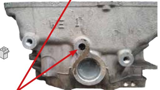
*If the injector seals or the rocker cover gasket are fitted incorrectly, oil will leak into the injector valley and out of this drain hole at the back of the head.*
