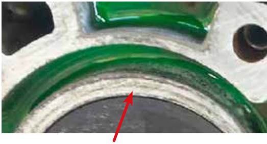
Fire ring surface rounded off with surface / whizzy discs
