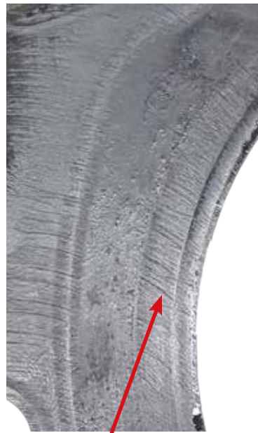
Marks in the head gasket are imprints of the deep scratches in the block caused by this.
