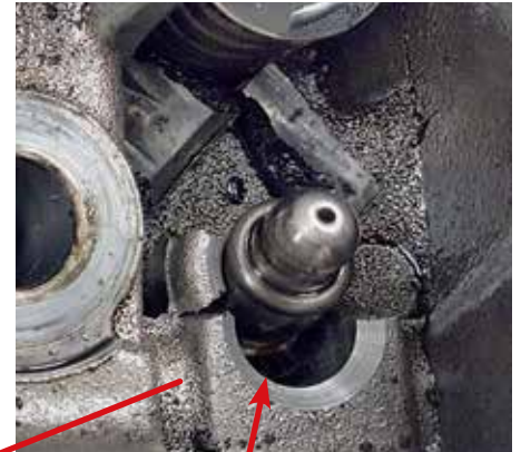
The valve lifters have been smashed out of the head due to the serpentine belt shredding, which caused the timing belt to fail.
