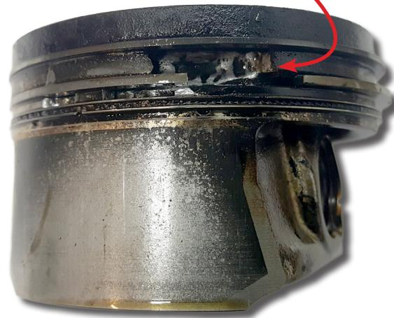
from the engine. If it occurs for a prolonged period, it will cause the ring lands to crack, the rings will break, which then start to wear their way through the ring lands (as shown in the pictures). The first signs of this problem will be some rough running, then misfire related codes, but by this time, the damage has been done. A compression test should be conducted to confirm the issue.
