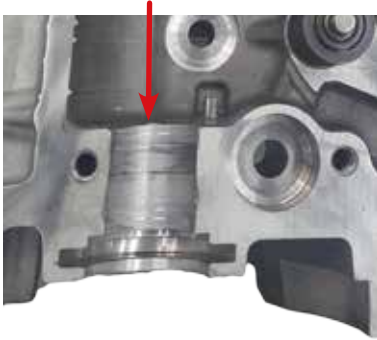
Front camshaft bearing surface in the head showing the signs of imminent seizure from lack of oil.
