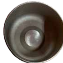
This bucket has been machined internally to allow clearance for the recessed valve.
