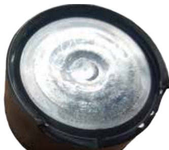
This shim's case hardening has been machined off which allowed the cam to wear a hole in it.
