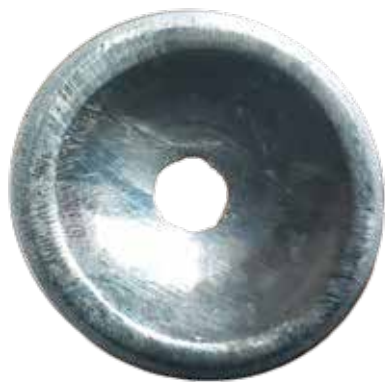
This shim's case hardening has been machined off which allowed the cam to wear a hole in it.
