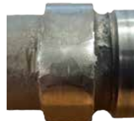
Causing the hardening to be worn off the cam lobes.
