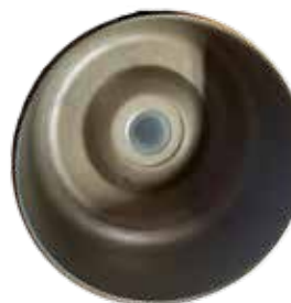
This is what a bucket should look like. Shims and buckets should NEVER be machined.
