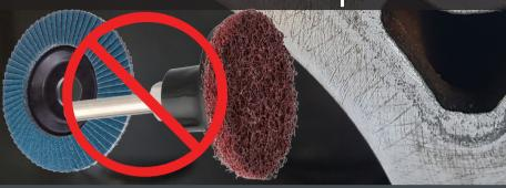
You can see the damage caused to the sealing surface of this cylinder block by a "Whizzy Disc" which has made the surface too rough. This would cause an MLS head gasket to fail.
