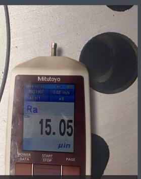
This is a block surface fresh of a surface grinder with a 15 RA surface finish as measured with a profilometer. You should aim for the closest to this as you can with sandpaper on a flat block.
