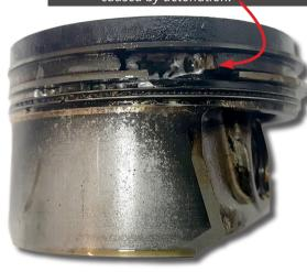
from the engine. If it occurs for a prolonged period, it will cause the ring lands to crack, the rings will break, which then start to wear their way through the ring lands (as shown in the pictures). The first signs of this problem will be some rough running, then misfire related codes, but by this time, the damage has been done. A compression test should be conducted to confirm the issue.
