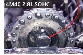
hexagon part of the camshaft. Do not use the timing chain to hold the camshaft as you could damage components or skip teeth. The torque specification for these camshaft bolts are:
